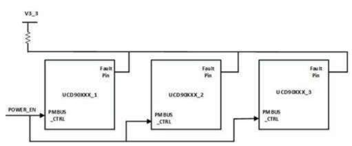
Figure 1. Example Using a Typical Fault Pin
