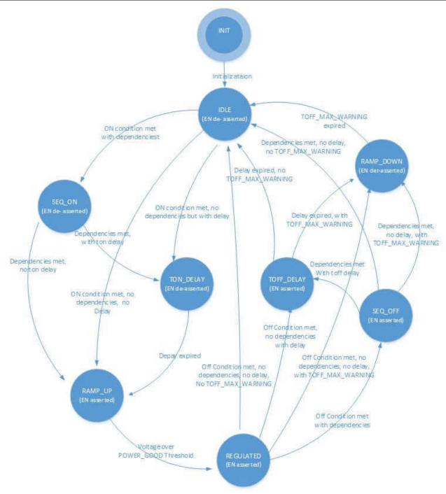
Figure 2. Rail State Machine Diagram
