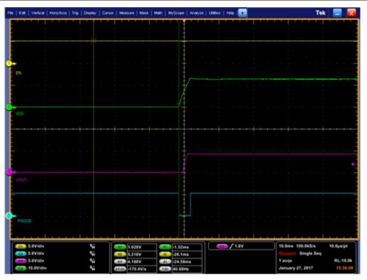
Figure 3. The TPS53315 Power-good Glitch That Results in PGOOD Ties to Enable: Enable Power Goes High First, Then VDD
