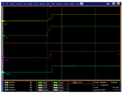
Figure 1. The TPS53315 Power Good Is Clean with No Glitches
