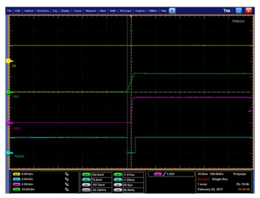
Figure 4. The TPS53319 Power-good Glitch That Results in PGOOD Ties to Enable: Enable Power Goes High First, Then VDD
