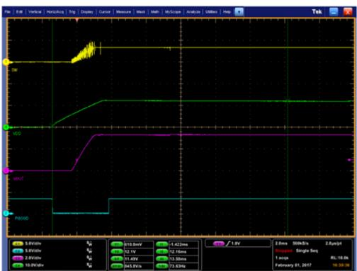
Figure 5. The TPS53319 Power-good Glitch That Results in an External 3.3V Pull-up on PGOOD Being Present before VDD/VIN
