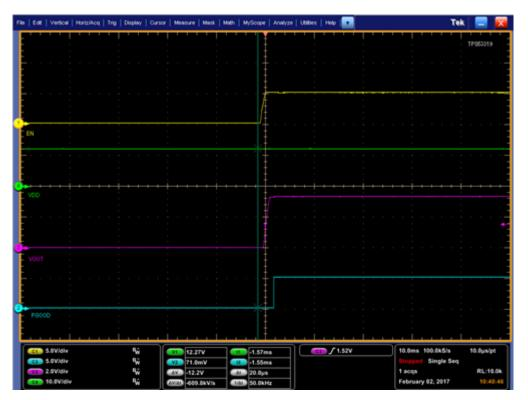
Figure 2. The TPS53319 Power Good Is Clean with No Glitches
