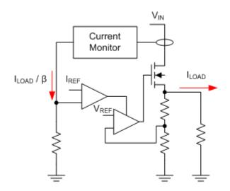
Figure 1. A Current-limiting Internal LDO Structure
