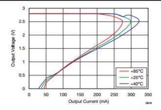
Figure 3. TLV717P Output Current Limit vs. VOUT
