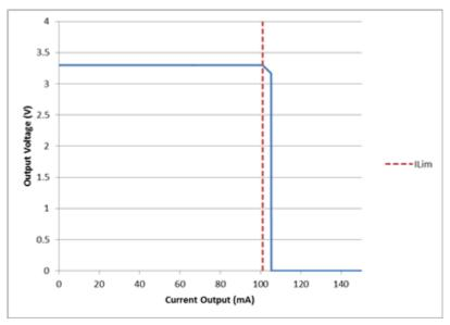
Figure 2. TPS7A16 Brick-wall Current Limiting (30VIN, 3.3VVIN, VSON at 25°C)
