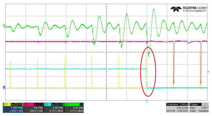
Figure 2. An TI LMG3410 Shoot-through Test on an LLC Series Resonant Half-bridge Converter: C1 = Low-side Switch Driving Signal, C2 = Switching-node Voltage, C3 = High-side Switch Driving Signal, C4 = Primary Inductor Current
