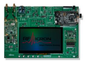
The Hermes platform is a unique, modular and scalable platform that reads the Smart Passive Sensors and performs critical processing; makes decisions and takes actions that are needed locally; and sends aggregated data to the cloud for longer term analytics. The platform incorporates an industry-standard Beaglebone Linux processor at its heart. This decouples the application and processing software from the specific hardware options and makes scaling processor power up or down a manageable task.
