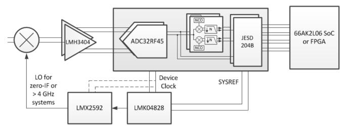
Figure 2. Direct RF Sampling Signal-chain Solution
