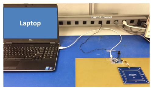
Figure 2. The Setup Consists of a Laptop, USB Cable, Custom Bezel Sensor, FDC2214 EVM and Large Ground Plane
