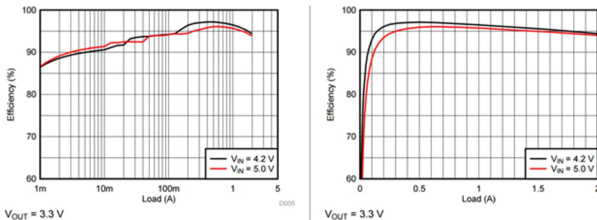
Figure 1. TPS62097 Efficiency with Power-save Mode (Left) and Forced PWM Mode (Right)
