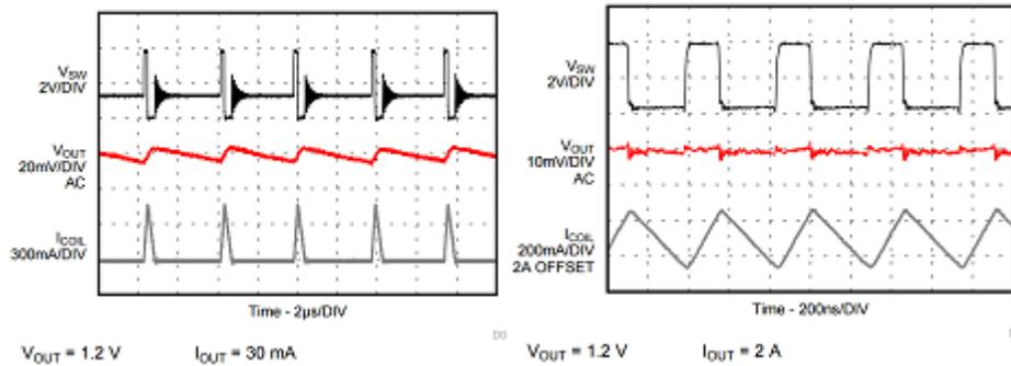
Figure 2. TPS62097 Output Ripple with Power-save Mode (Left) and Forced PWM Mode (Right)
