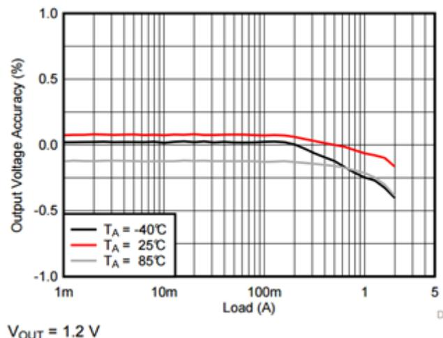
Figure 3. Output-voltage Accuracy over Temperature and Load
