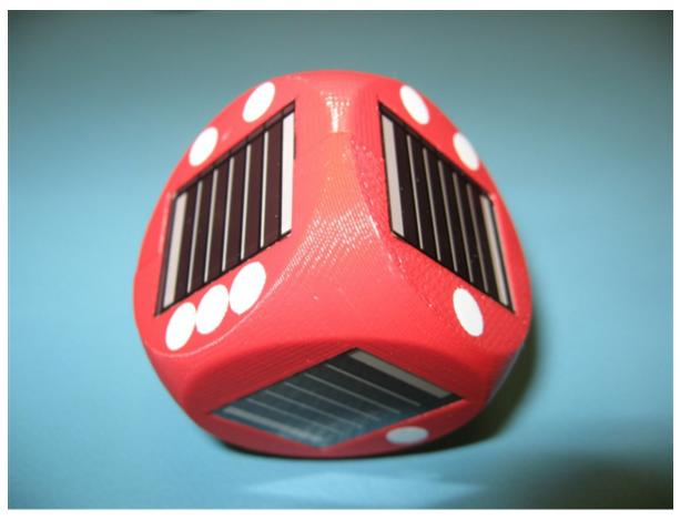
Figure 1. The Solar Dice Is an Example of an IoT Sensor Node
