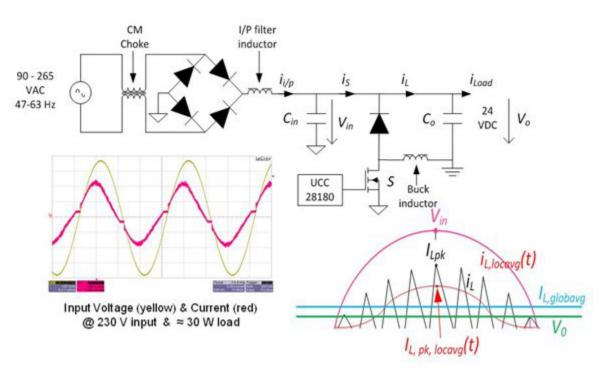
Figure 3. Circuit Diagram of the Buck PFC Topology
