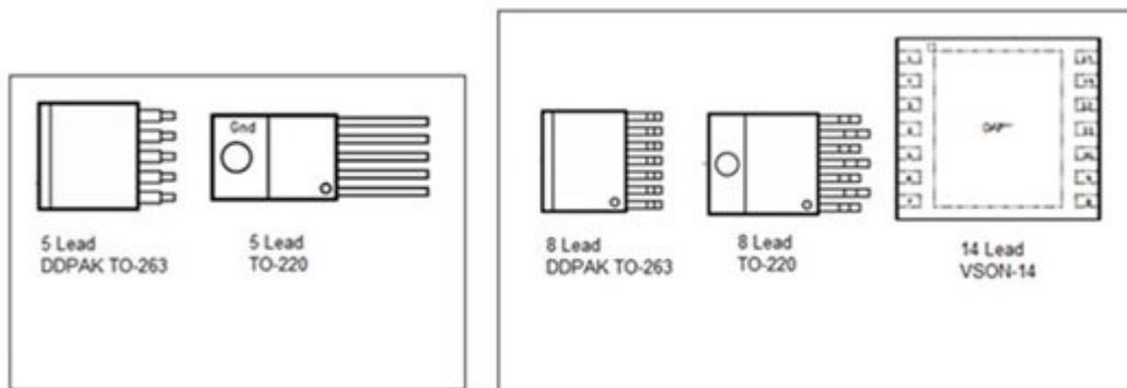
**Figure 1. LM2576, LM2596, and LM2676 Regulators**
