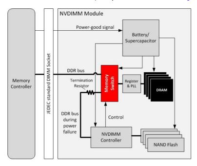
Figure 1. Using a Memory Switch in NVDIMM Application
