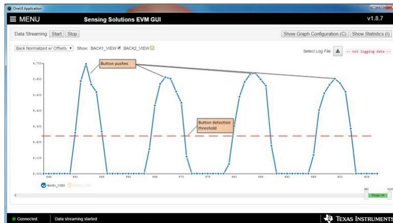
**Figure 3. LDC1612 Output Response with Four Button Pushes**
