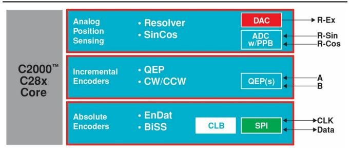
The F28379 MCUs are the first commercial microcontrollers offering the breadth of position sensor support, flexibility, scalability and robustness to make the need for custom FPGA support a thing of the past. Solutions for these four sensors as well as incremental encoders are included at no charge as part of the controlSUITE™ software suite.
