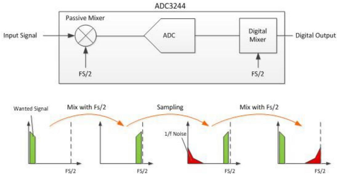
**Figure 2. Chopper Implementation Details of the [ADC3244](#)**
