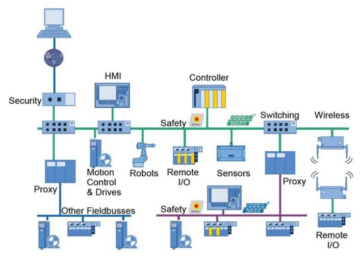
Figure 1. PROFINET Network in an Automation System
