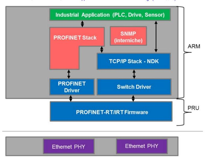
Figure 4. PROFINET RT/IRT Solution on Sitara Processors
