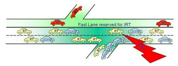
Figure 3. Profinet Irt Fast Lane
