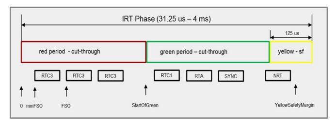
Figure 2. PROFINET IRT Communication Phase
