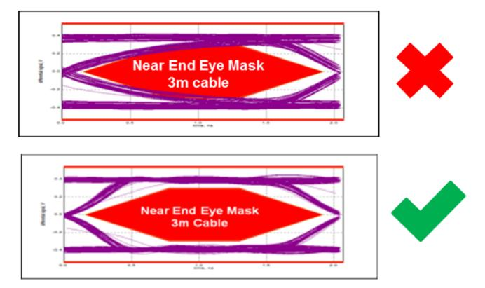
Figure 1. The TUSB211 Improves the Raising Edge in a Near-side Eye Mask with a 3m Cable
