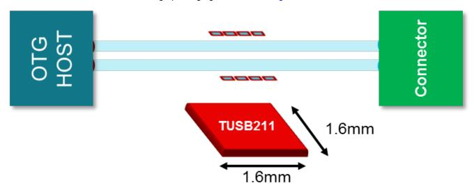
Figure 2. The TUSB211 Is Designed onto a Printed Circuit Board (PCB) without Populating the Device to Enable Easy Modifications
