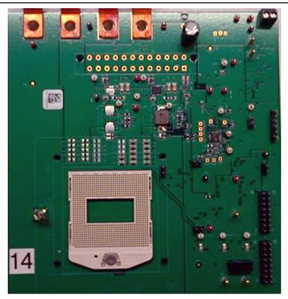
Figure 2. TPS51623 Intel Braswell (Pentium N3700) Reference Design.
