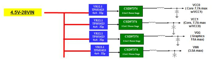
Figure 1. TPS51623 Vcore Controller Powers Intel's Braswell Processor.
