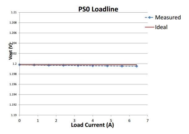
Figure 3. TPS51623 Reference Design CPU Loadline (Load Regulation) Data.
