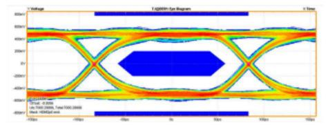
Figure 1. HDMI 2.0 Test Point 1 (TP1) Eye Diagram of TPD4E05U06 ESD Protection Device
