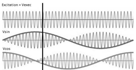
Figure 2. Waveform across the Resolver Coils
