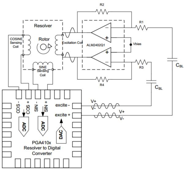
Figure 3. The ALM2402 In a Resolver Application
