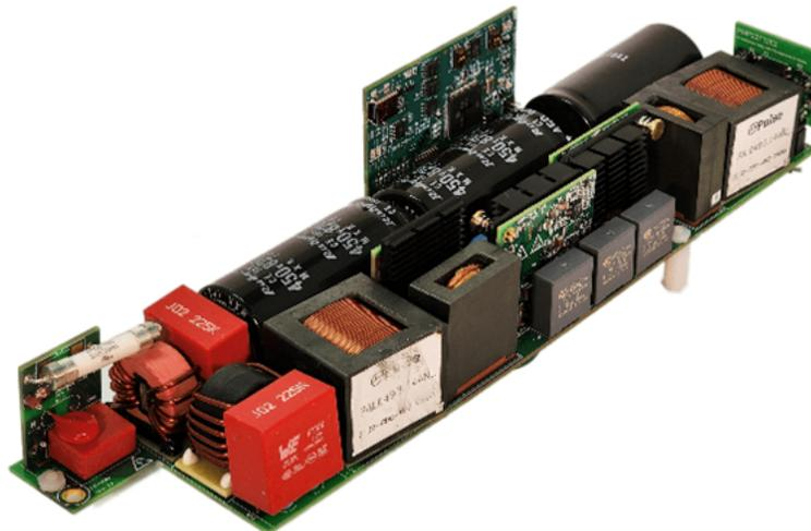
Figure 4. A 400-V, 5-kW prototype with a power density of 120 W/in<sup>3</sup>.
