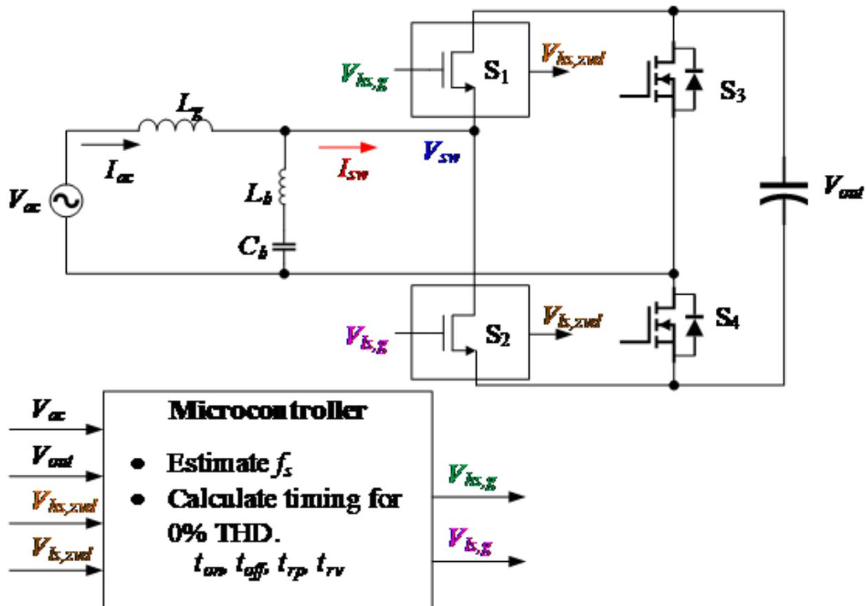
Figure 2. A single-phase iTCM schematic with control signals.
