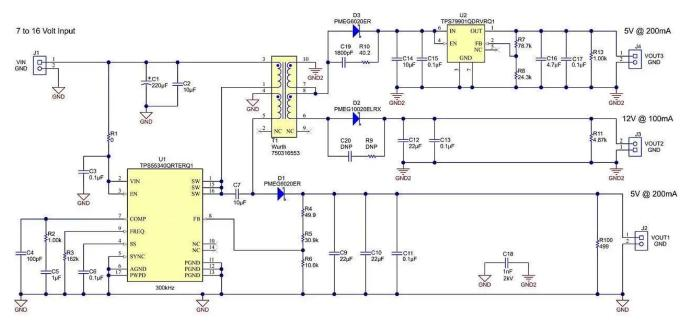
Figure 3. Actual SEPIC design with dual isolated outputs.
