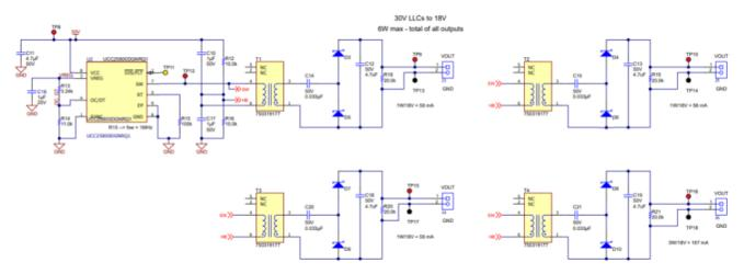
Figure 1. From the pre-regulated reference design schematic—the isolated four-output converter. Source: Texas Instruments
