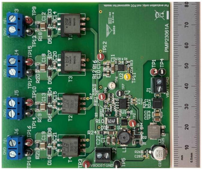
Figure 2. Pre-regulated reference design assembled board, including boost circuit from 6 V<sub>IN</sub>. Source: Texas Instruments
