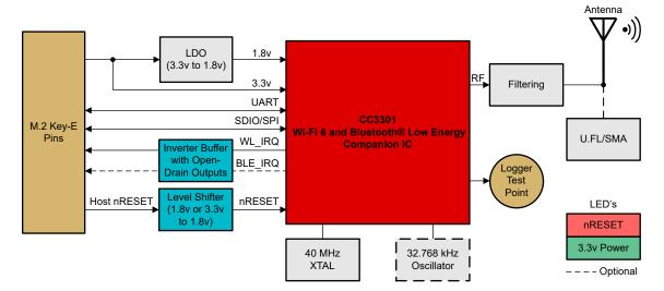
Figure 1-1. Block Diagram of M.2-CC3301
