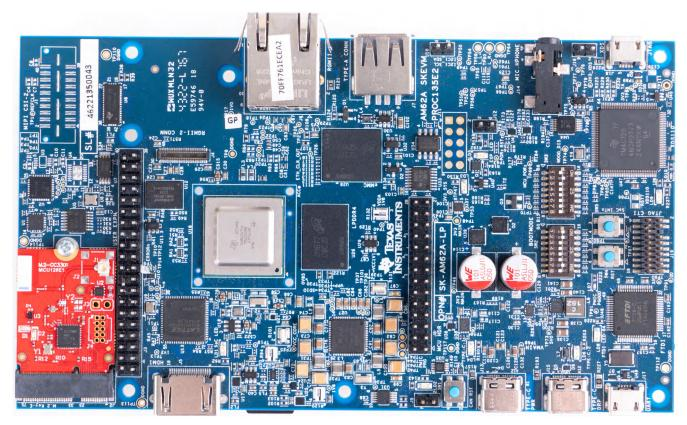
Figure 2-3. M2-CC3301 on SK-AM62A-LP
