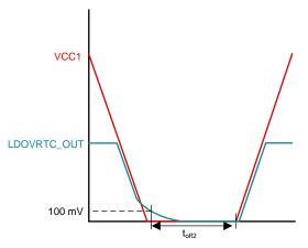
Figure 4. LDOVRTC Discharge With Resistor
