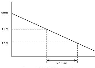
Figure 1. VCC Falling Profile
