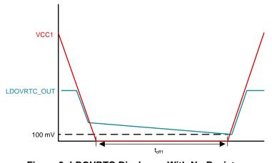
Figure 3. LDOVRTC Discharge With No Resistor
