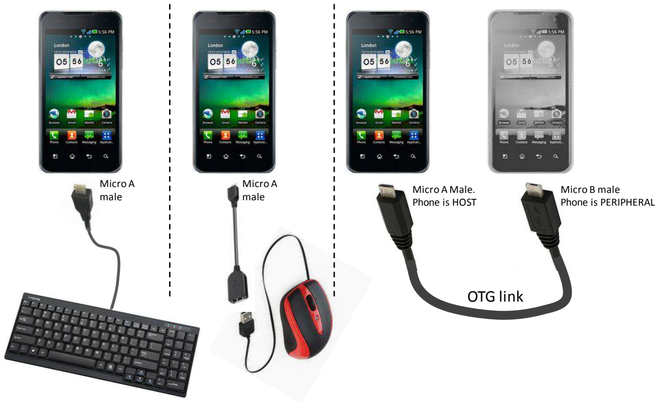
Figure 5. Smart Phone With the OMAP4 USB OTG Device Used as Host
