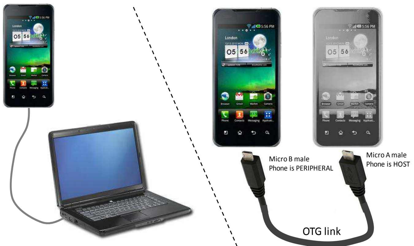
Figure 2. Smart Phone With OMAP4 USB OTG Used as Peripheral
