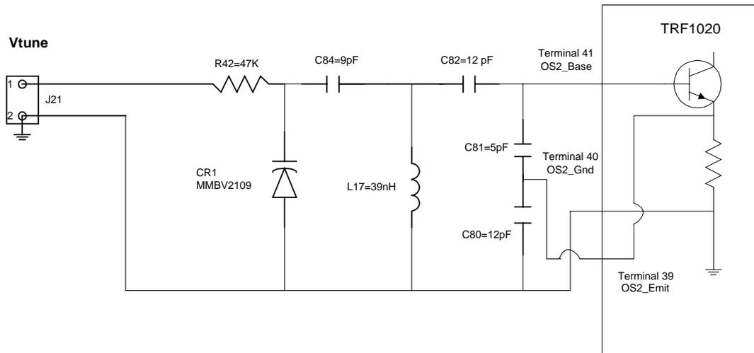
NOTE: The tank circuit in Figure 2 has been redrawn in Figure 4 for clarification.
