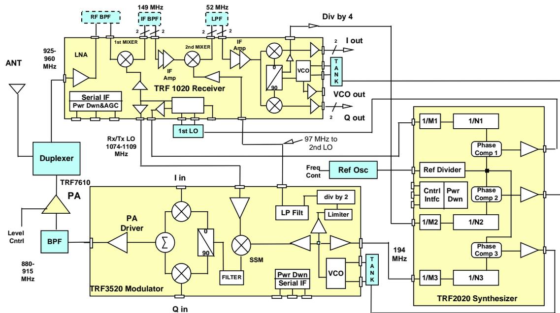
The TRF1020 is used in conjunction with the TRF3520 Modulator, the TRF2020 Synthesizer, and the TRF7610 Power Amplifier to create a complete GSM solution.
