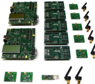
2 x SmartRF05EB (the large boards)
