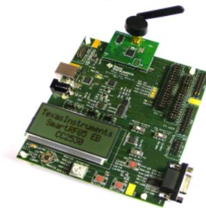
Make sure that P14 (the RS232 switch) is set in position *Enable* on this board.
