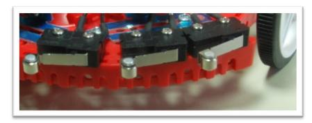
Figure 1. Bump sensors positioned at the front of the robot.
