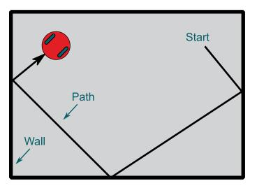
Figure 2. A possible integrated maze is to explore inside a box.
