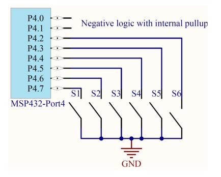
Figure 4. One possible interface circuit for the bump sensors. Using Port 4, will conflict with the CC3100/CC3120 wifi module. However, only Ports 1 - 6 can trigger interrupts.
