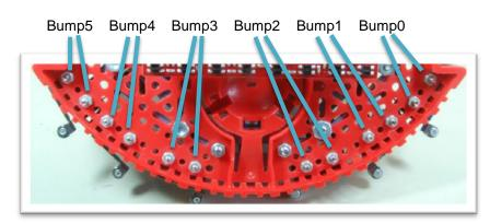
Figure 3. Bump sensors attached to the front of the robot (bottom view).
