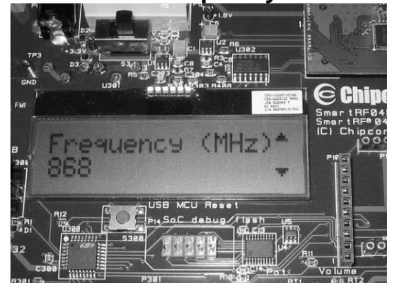
Select frequency according to the type of EM module in use (315 MHz, 433 MHz, 868 or 915 MHz). Move the joystick up or down to display the choices and push button S1 in the lower right corner of the board to select the displayed frequency.
