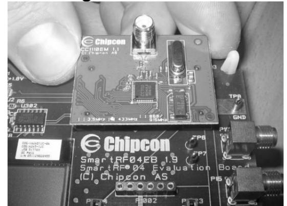
Insert a CC1110EM into both SmartRF04EBs. The connectors will only fit in one position, so that the EM cannot be inserted the wrong way. Do not force the EM.
