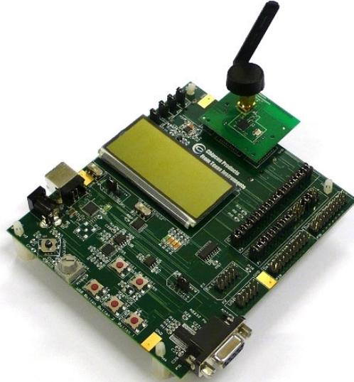
**Figure 11 - CC2520EM connected to SmartRF05EB**
