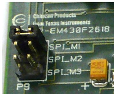
**Figure 23 - SPI Mode selection header**
