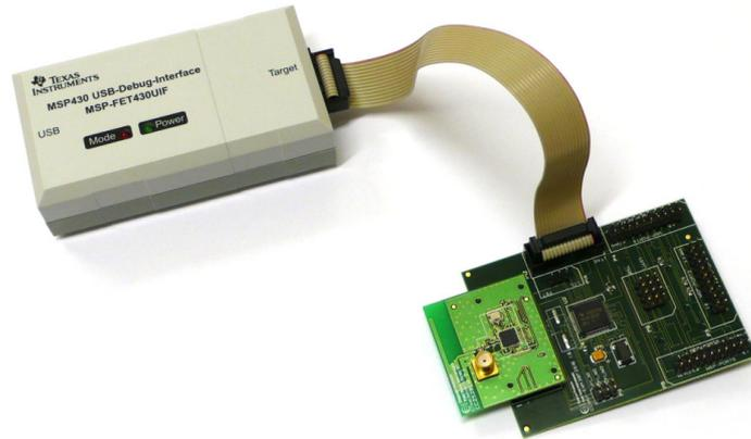
**Figure 9 - EM and MCU board operating standalone**
