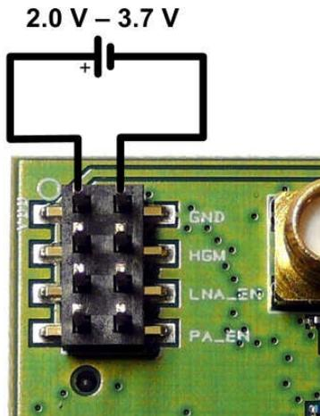
**WARNING: Do not connect a jumper between P5 pins 1-2, as this will short-circuit the power supply!**
