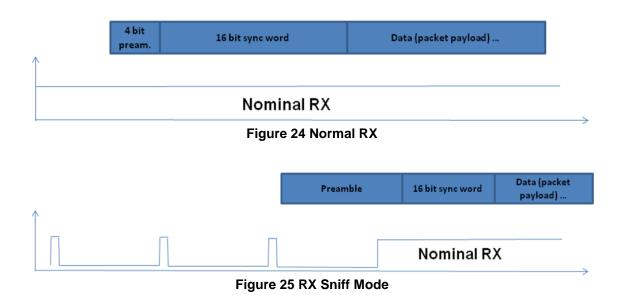
The configuration uses 1.2 kbps data rate with 4 byte preamble. In this example the average current consumption when the radio is duty cycling is measured to 1.9 mA opposed to 25.1 mA which is the current consumption when the receiver is set in continuous RX.
