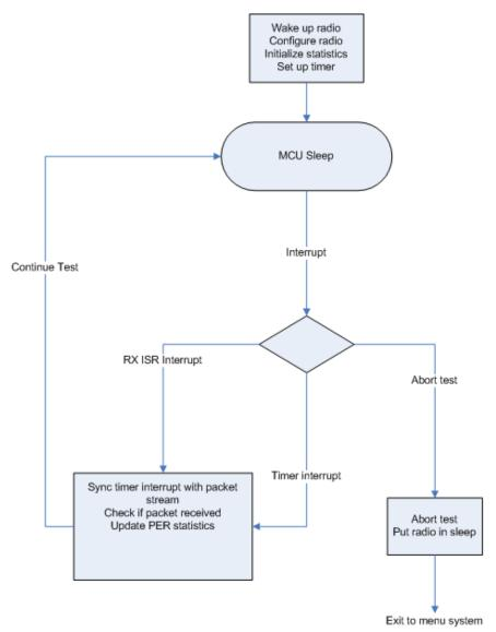
Figure 16 One-way PER test at Master
