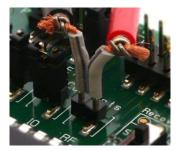
**Figure 32 Current measurement**
