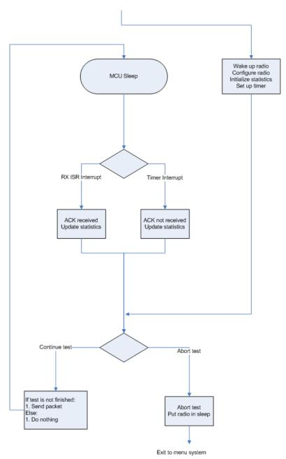
Figure 18 Two-way PER test at Master
