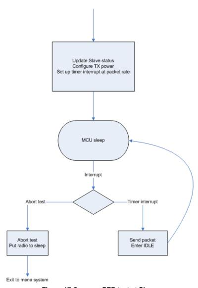
Figure 17 One-way PER test at Slave
