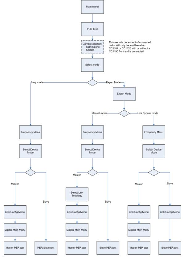
Figure 6 PER test Menu Tree
