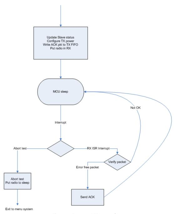
Figure 19 Two-way PER test at Slave
