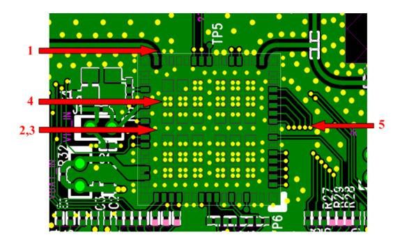
Figure 18. Module Layout Guidelines (Top Layer)
