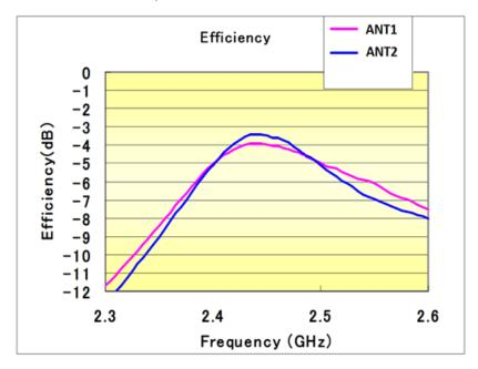
Figure 5. Antenna Efficiency
