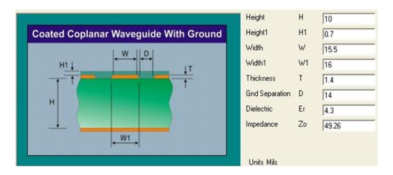
Figure 20. Trace Design for the PCB Layout
