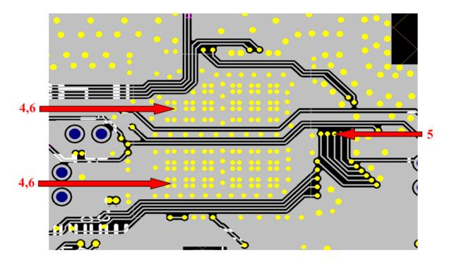
Figure 19. Module Layout Guidelines (Bottom Layer)
