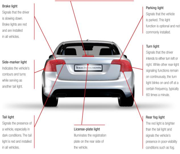
Figure 1. Components of a rear-lighting system.
