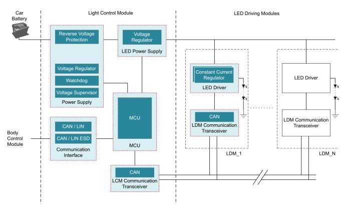
Figure 6. A digital interface LED driving module architecture for pixelated rear lights.
