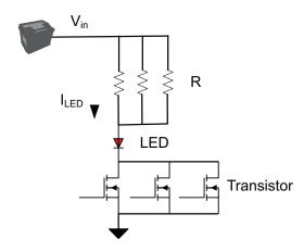
Figure 9. Discrete LED driver.
