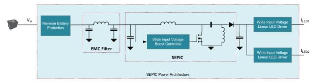
Figure 8. Dual-stage LED driver.
