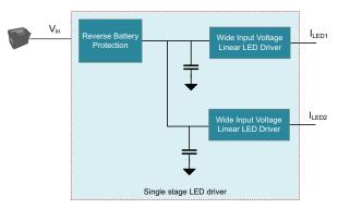
Figure 7. Single-stage LED driver.
