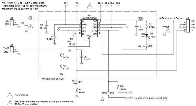
Apply Shunt JP3 to connect Pulse Generating Hardware.
