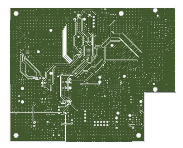
TEXAS INSTRUMENTS, INC. ADC16DX370/LM97937 EVM PCB REV A LAYER 4- GROUND PLANE 2
