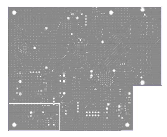
TEXAS INSTRUMENTS, INC. ADC16DX370/LM97937 EVM PCB REV A LAYER 2- GROUND PLANE 1
