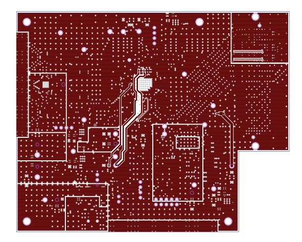
TEXAS INSTRUMENTS, INC. ADC16DX370/LM97937 EVM PCB REV A LAYER 3- POWER PLANE
