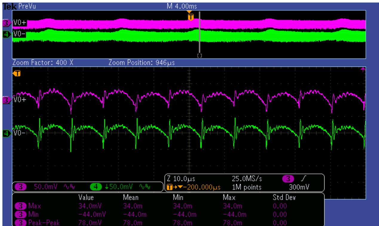
The output ripple voltage is shown in the figure below. The image was taken with the  $\pm 42\text{V}$  output loaded to 6A and the input voltage set to 220VAC. (CH3: +42V output in AC coupling, CH4: -42V output in AC coupling)
