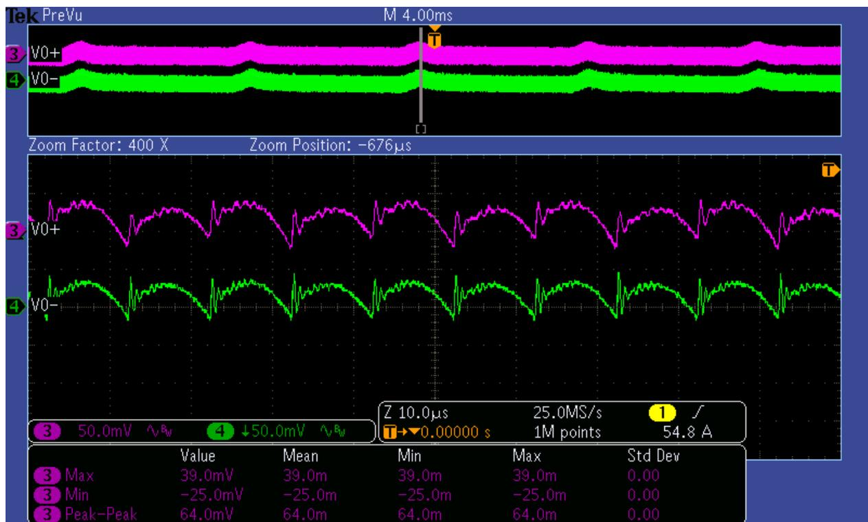
The output ripple voltage is shown in the figure below. The image was taken with the  $\pm 42\text{V}$  output loaded to  $0\text{A}$  and the input voltage set to  $110\text{VAC}$ . (CH3:  $+42\text{V}$  output in AC coupling, CH4:  $-42\text{V}$  output in AC coupling)
