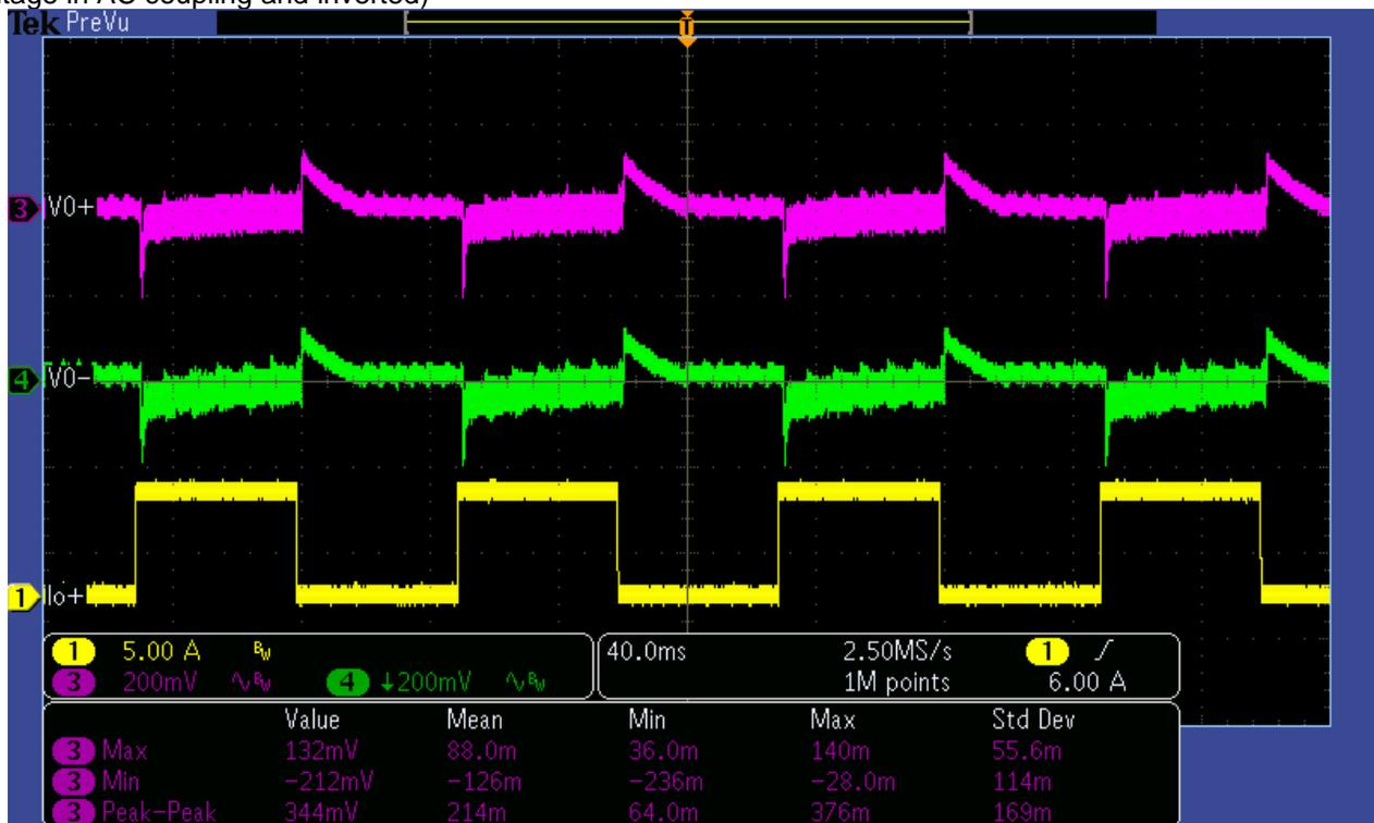
The photo below shows the  $\pm 42\text{V}$  output voltage when the load current is stepped between 6A and 12A with an input voltage of 110VAC. (CH1: +42V output current, CH2: -42V output current, CH3: +42V output voltage in AC coupling, CH4: -42V output voltage in AC coupling and inverted)
