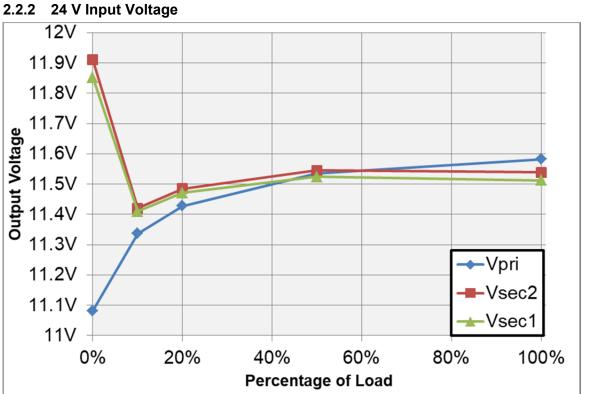
Figure 5. Output Voltage vs Load for the 11 V Outputs
