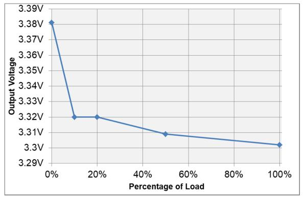
Figure 8. Output Voltage vs Load for the 3.3 V Output
