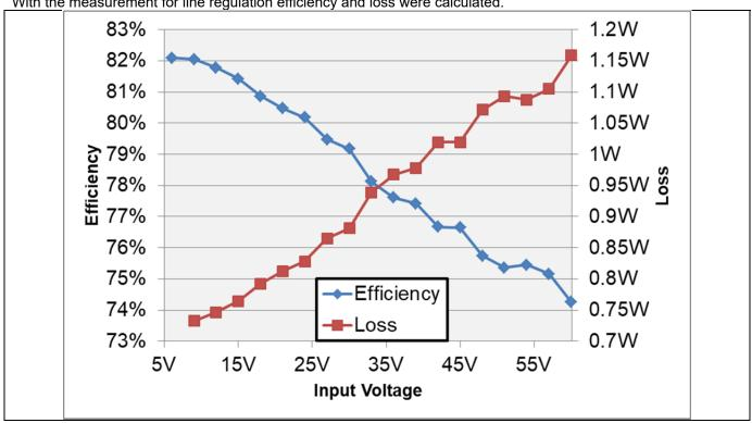
With the measurement for line regulation efficiency and loss were calculated.
