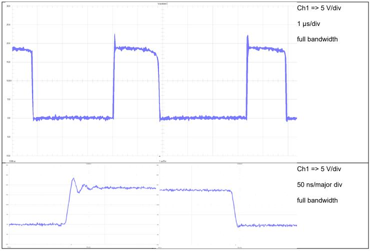
Figure 15 Switchnode to GND @ 6 Vin
