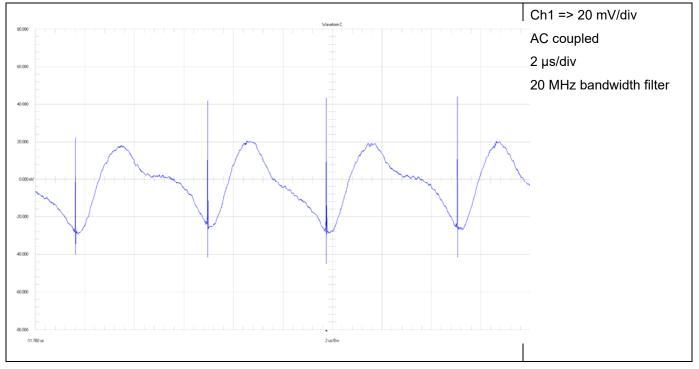
Figure 26. Input Voltage Ripple 6 V
