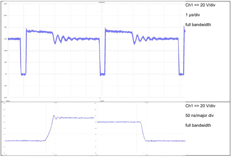
Figure 17 Switchnode to GND @ 60 Vin SEPIC
