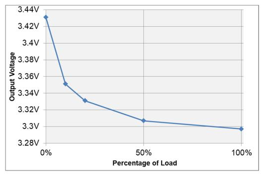
Figure 4. Output Voltage vs Load for the 3.3 V Output
