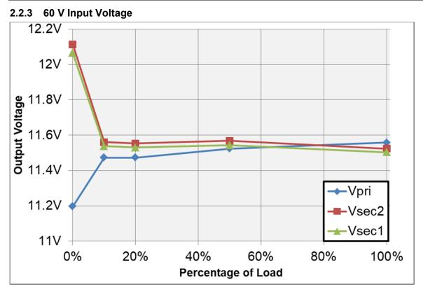
Figure 7. Output Voltage vs Load for the 11 V Outputs
