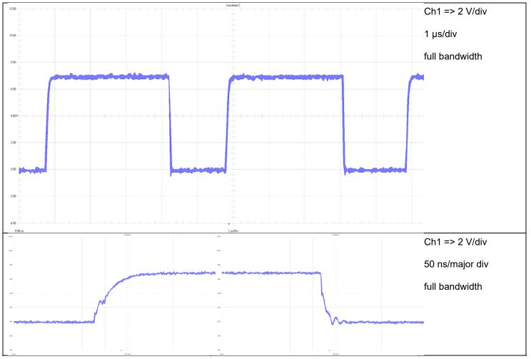
Figure 19 Gate to GND @ 6 Vin
