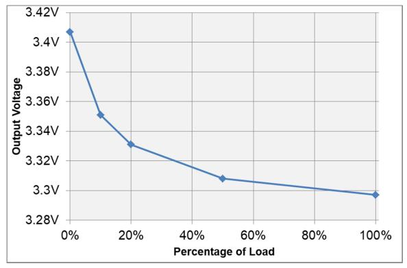
Figure 6. Output Voltage vs Load for the 3.3 V Output
