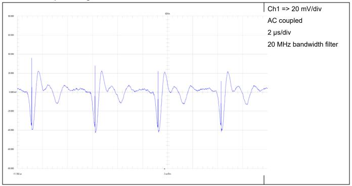
Figure 28. Input Voltage Ripple 60 V
