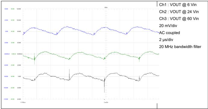
Figure 25. 11 V Output Voltage (Isolated Vo2)
