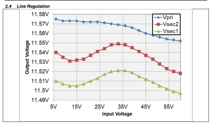
Figure 9. Output Voltage vs Input Voltage for the 11 V Outputs
