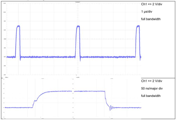
Figure 21. Gate to GND @ 60 Vin
