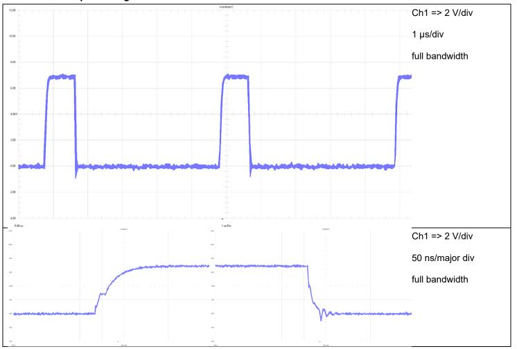
Figure 20. Gate to GND @ 24 Vin
