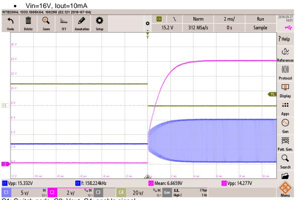
C1: Switch node, C2: Vout, C4: enable signal
