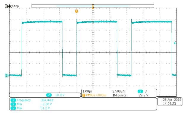
• Ch1: Switching node at 36.0V in and 2.0A load current [scale: 10.0V/div, 1.0us/div]
