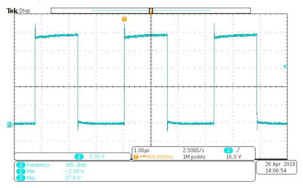
• Ch1: Switching node at 12.0V in and 2.0A load current [scale: 5.0V/div, 1.0us/div]
