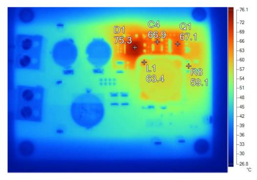
Thermal image of the PCB's top side at 12.0V in and 2.0A load current. Thermals can be improved by using a larger diode package and larger cooling areas.
