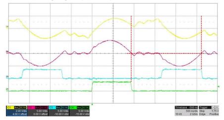
2.4.4 F<sub>sw</sub>=500kHz, 3kW: C1: XFMR Primary Winding Current (100mV/A), CH2: XFMR Secondary Winding Current (200mV/A), CH3: SR Driving Signal (PWM3A), CH4: SR Driving Signal (PWM3B)
