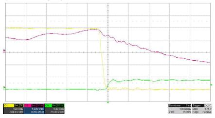
2.4.2 Soft-switching waveforms at 566Vprim, 420Vsec/3.3kW – 700kHz: C1: Primary LS FET VDS, C2: XFMR Primary Winding Current (100mV/A), C4: PWM2B – Primary LS FET Driving Signal.
