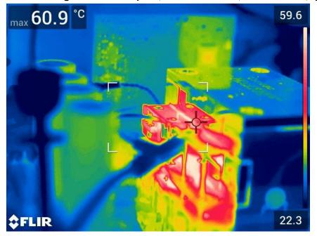
2.3.1 Charge mode: 383Vprim, 280Vsec/6.6kW, Fsw=508kHz, n=96.93%
