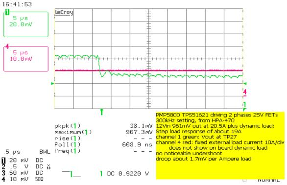
Step load response using 'on board" dynamic load: 13-Jul-10
