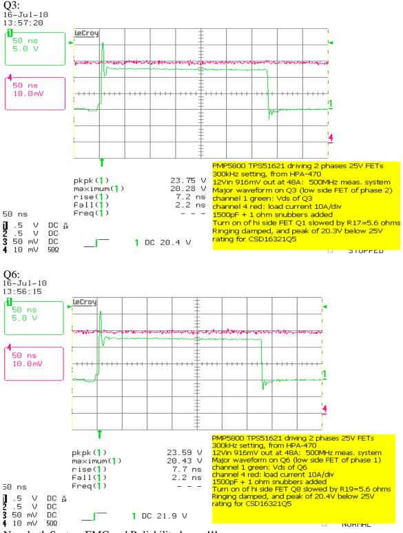
Finally, the gate drive to the high side FETs were slowed with R17 and R19 increased to 5.6 ohms from zero. This change only slows turn on, not turn off of hi side FETs.
