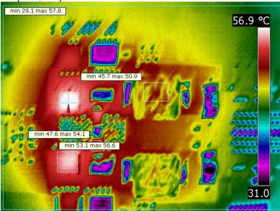
Thermal summaries for these two runs shown below at full 48A load with and without airflow. See the full Thermal Report in .pdf form for PMP5800 to see the actual images:
