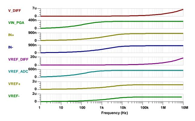
Figure 16. Simulated Noise Performance (y-axis is in Vrms)
