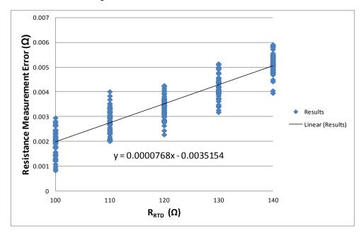
Figure 19. Resistance Measurement Results with Precision Resistors before Calibration
