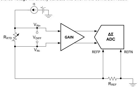
Figure 3. Ratiometric RTD Measurement
