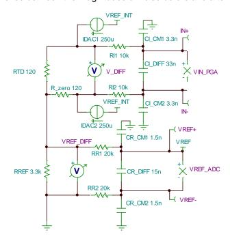
Figure 15. Noise Performance Simulation Schematic
