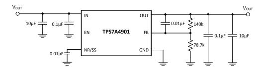
Figure 10. LDO Configuration for +3.3 V Output
