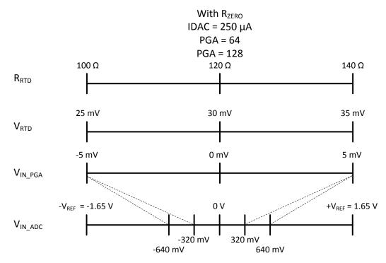
Figure 7: ADC Input Signals in a Hardware Compensated System
