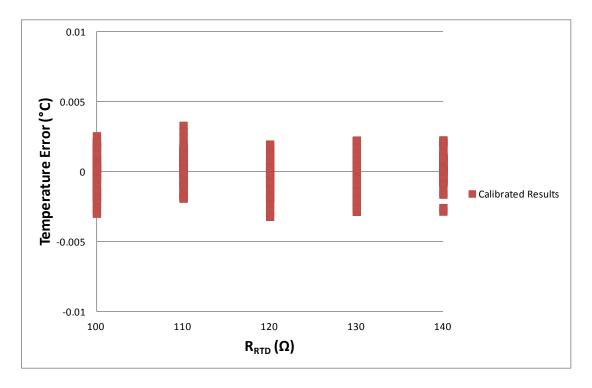
Figure 1. Measured Temperature Accuracy with Resistive Input Representing 0°C - 100°C
