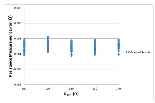
Figure 20. Resistance Measurement Results with Precision Resistors after Calibration
