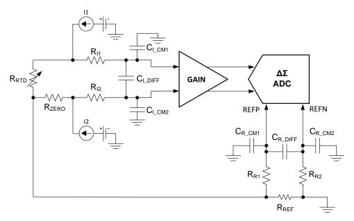
Figure 8: Input and Reference Low-Pass Filtering
