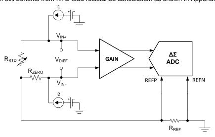
Figure 5. Hardware Compensated 3-Wire RTD System
