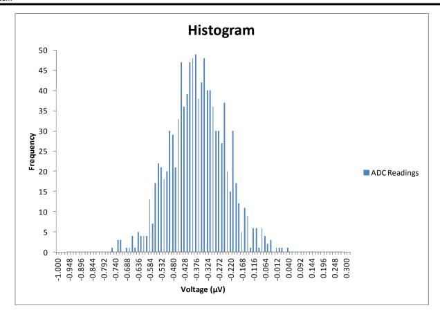
Figure 22. Histogram with  $R_{RTD} = 120 \Omega$ , 0.01%
