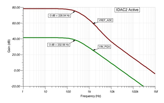
Figure 28. Input Filter Frequency Response with IDAC2 Active
