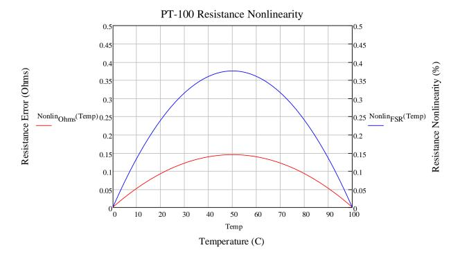
Figure 26. PT-100 RTD Non-Linearity from 0°C - 100°C
