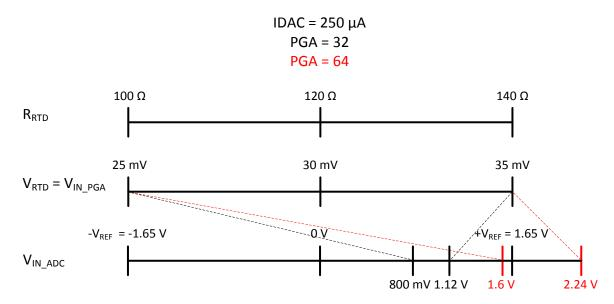
Figure 6: ADC Input Signals in a Traditional RTD System
