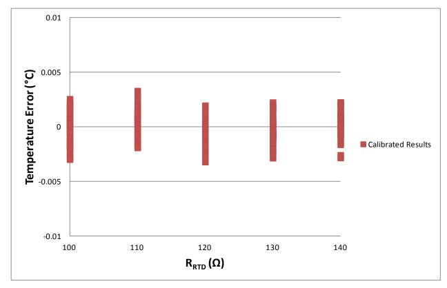
Figure 21: Calculated Temperature Error from Resistance Measurement Error
