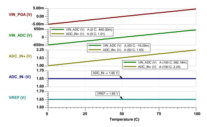
Figure 13. The Input and Output of the PGA and VREF from 0°C - 100°C
