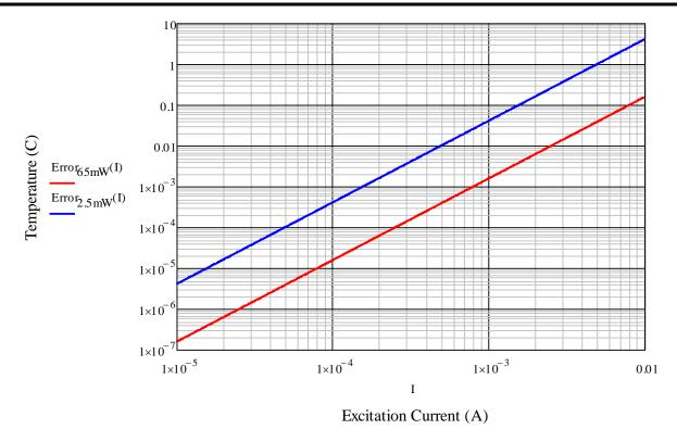
Figure 4: RTD Self-Heating vs. Excitation Current for Different RTD Types
