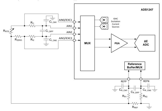
Figure 9: Hardware Compensated Ratiometric RTD System Featuring the ADS1247
