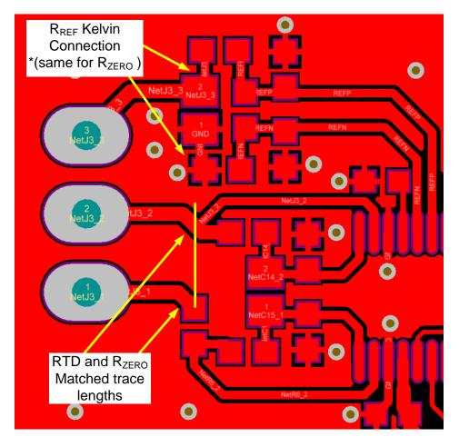
Figure 17. PCB Layout Highlighting Important PCB Layout Concerns
