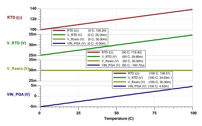
Figure 12. RTD, R<sub>ZERO</sub>, and PGA Input from 0°C - 100°C
