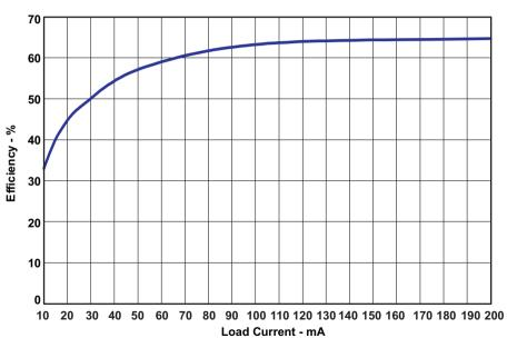
Figure 4. Efficiency Over Load Current
