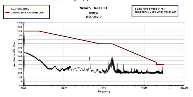
Figure 3. Radiated Emissions (dBµV/m) from 10 kHz to 30 MHz
