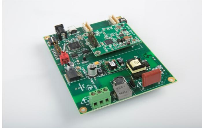
**Figure 4. Dock + SOMPLC-F28PLC83 Module Plugged**
