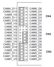
Figure 1 Header configuration for 4 camera, 12 bits per camera
