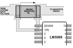
Figure 17. U1 SENSE and  $V_{IN}$  Pin Pad Connection using Resistors of Kelvin Type
