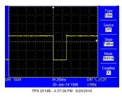
Figure 12. Output Voltage of the Protection Device during Surge at 100- $\Omega$  Load
