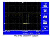
Figure 14. Output Voltage of the Protection Device during Surge at 15- $\Omega$  Load
