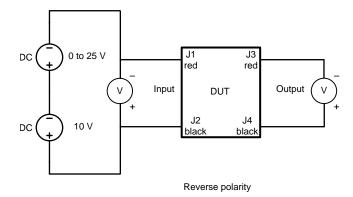
Figure 6. Measurement Setup for Reverse Polarity Current Measurement
