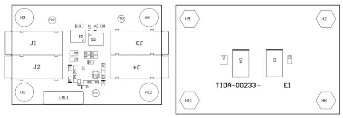
Figure 28. Top Assembly Drawing
