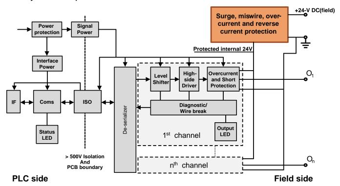
Figure 1. Use of This Design (Orange Block) in System Context (High Side Driver with 24-V Field Supply)
