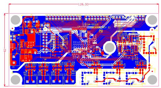
Figure 22. Multilayer Composite Print
