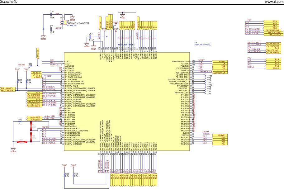
Figure 20. Schematic - MSP430F6779 + Crystal
