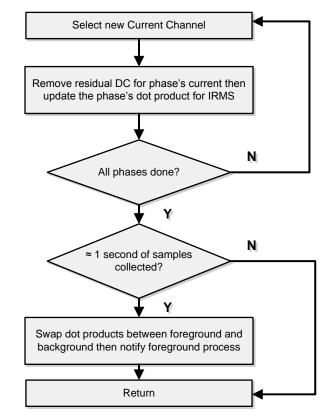
Figure 9. per\_sample\_dsp() Function
