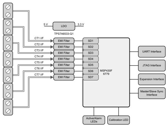
Figure 1. Block Diagram of BCM Module
