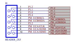
Figure 6. SPI / I2C / UART Expansion Interface
