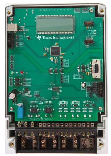
Figure 11. Top View of the Energy Meter EVM
